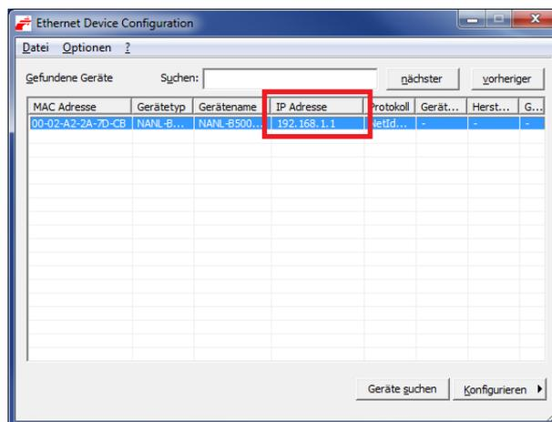
Figure 19: Ethernet Device Configuration - NANL-B500G-RE found (Example)
