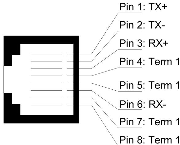
Figure 28: Ethernet pinning at the RJ45 socket
