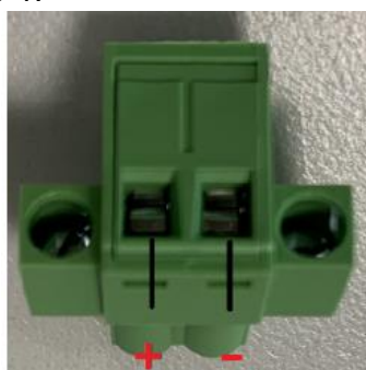
Figure 2.1 Power Connector and Power Lines
