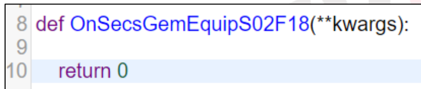
Figure 4-309 Add the OnSecsGemEquipS02F18 function in the script editing area
