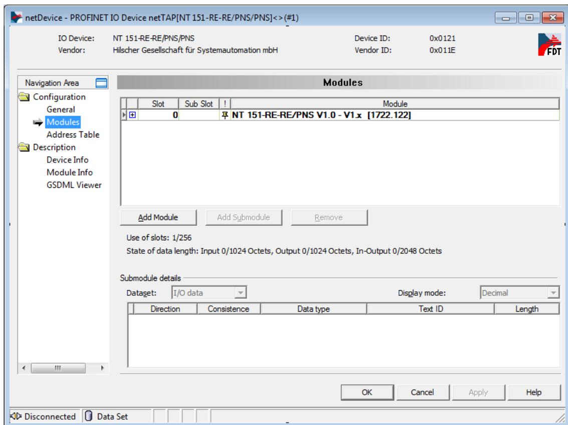
Figure 61: Configuring PROFINET IO Device at X2 (1)
