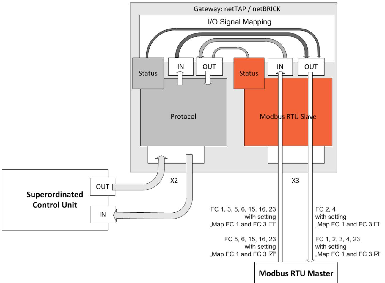
Figure 154: Access from the Modbus RTU Master to the netTAP and netBRICK Device
