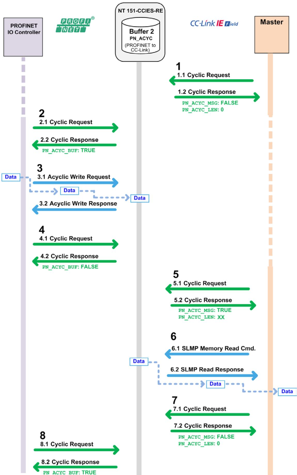
Figure 169: Sequence of Acyclic Communication of PROFINET to CC-Link IE Field
