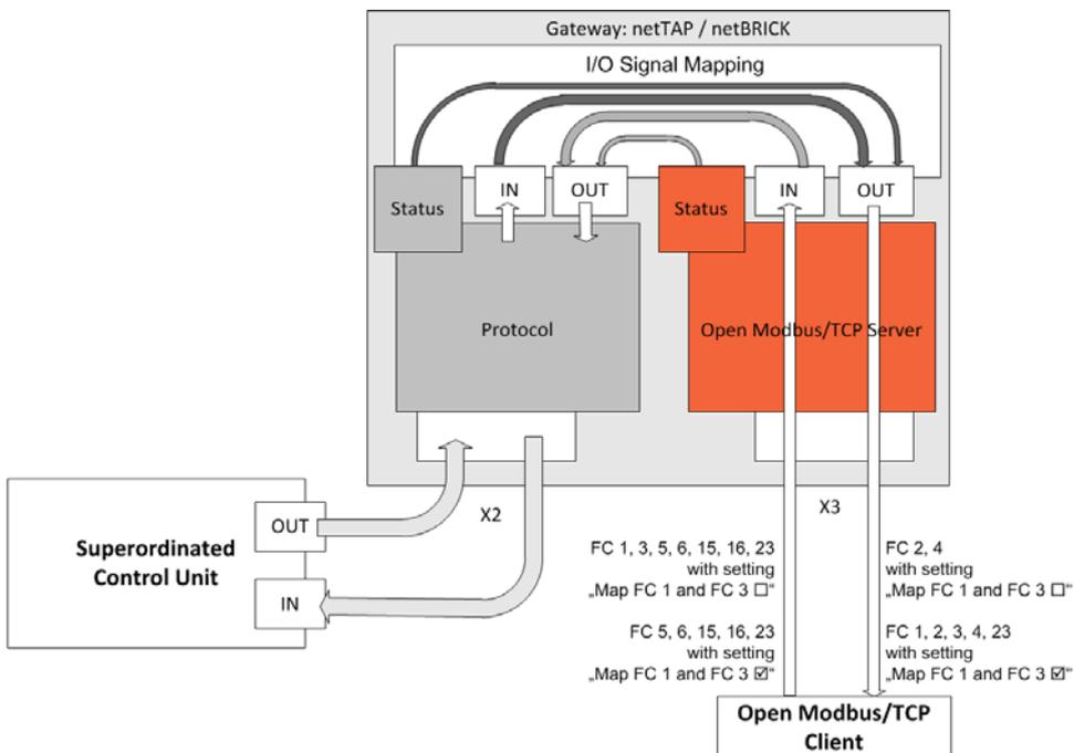
Figure 149: Access of the Open Modbus/TCP Client to the netTAP and netBRICK Device
