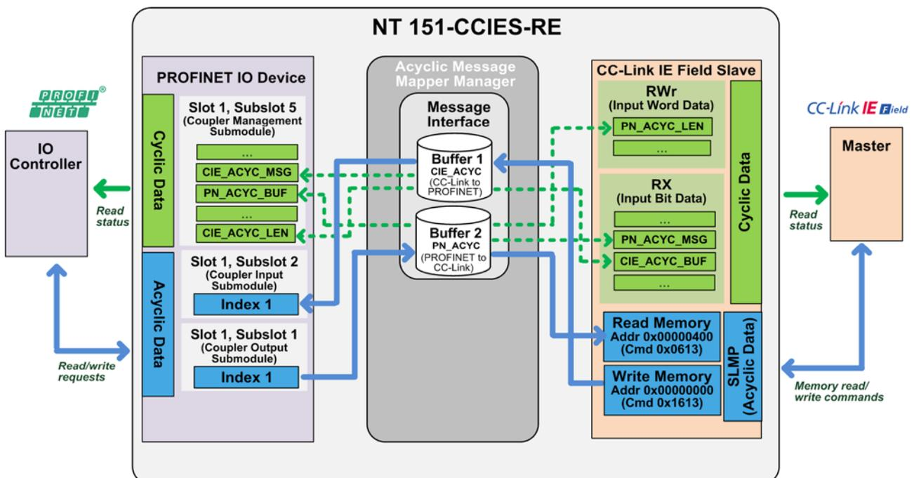
Figure 168: Acyclic Communication via Message Interface Buffer
