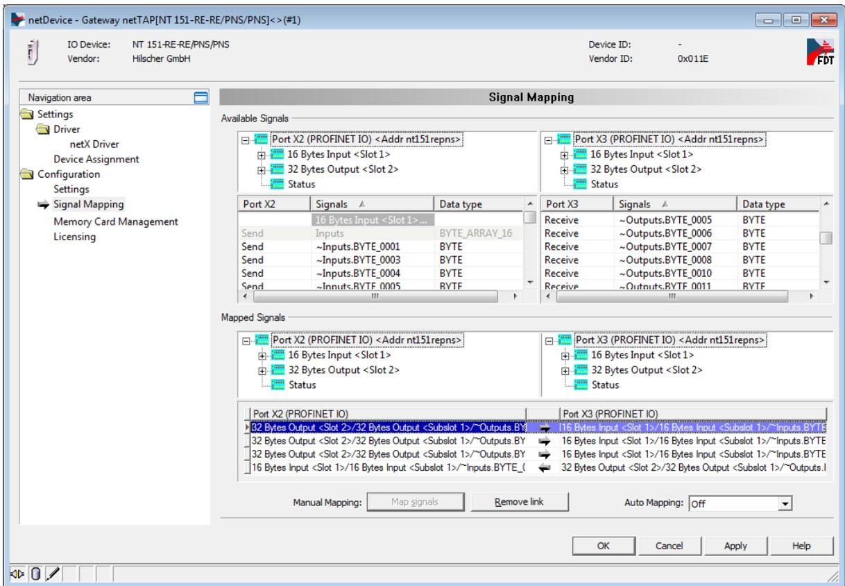
Figure 73: Gateway Signals mapped
