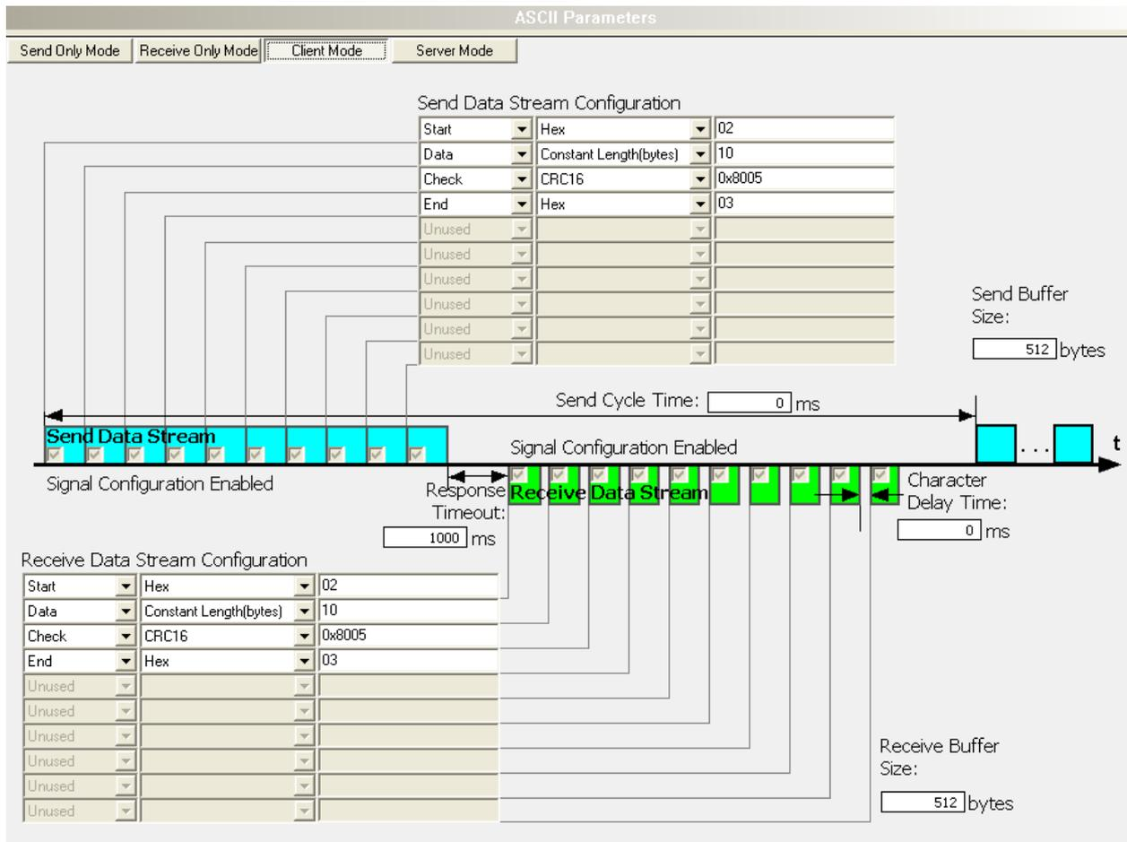
Table 77: Telegram Structure for the Operating Mode 'Client Mode'
