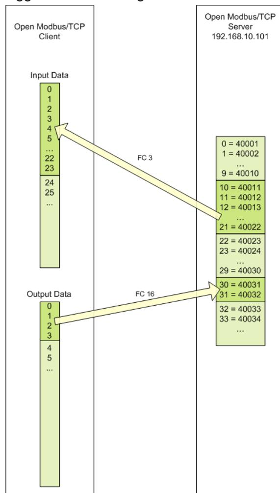
Figure 148: Examples - Reading Command with FC 3, Writing Command with FC16
