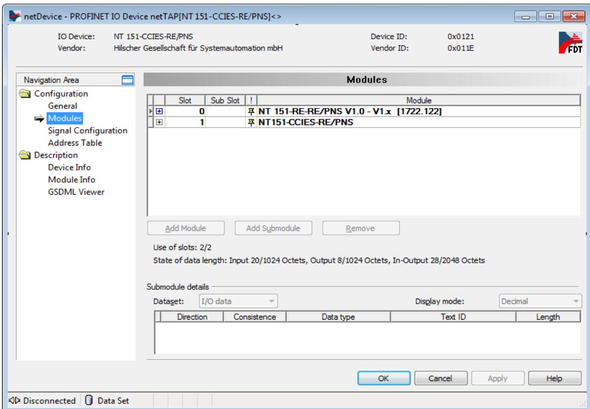
Figure 92: Configuration dialog PROFINET Device
