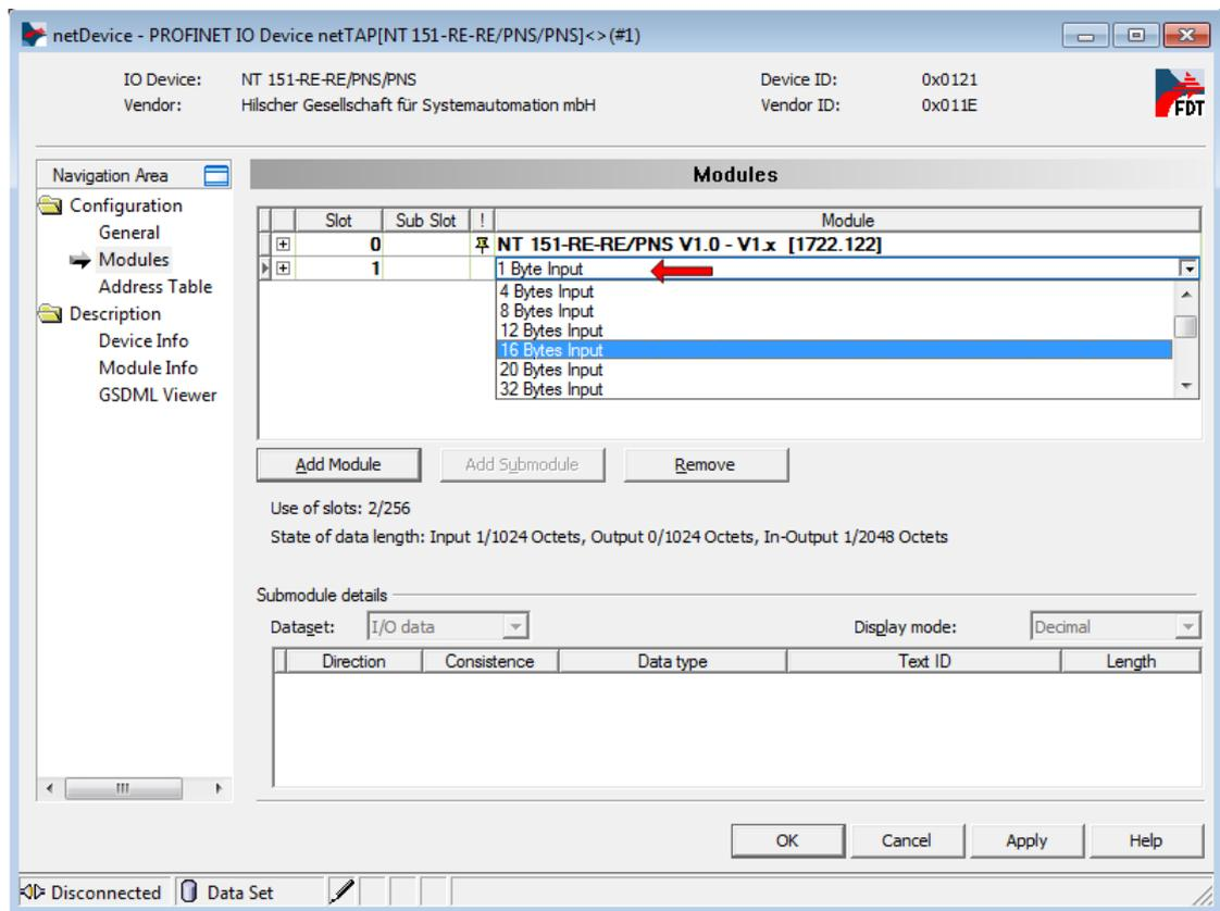
Figure 66: Configuring PROFINET IO Device at X3 (1)
