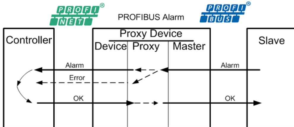
Figure 160: PROFINET IO- PROFIBUS DP – Alarm Errors
