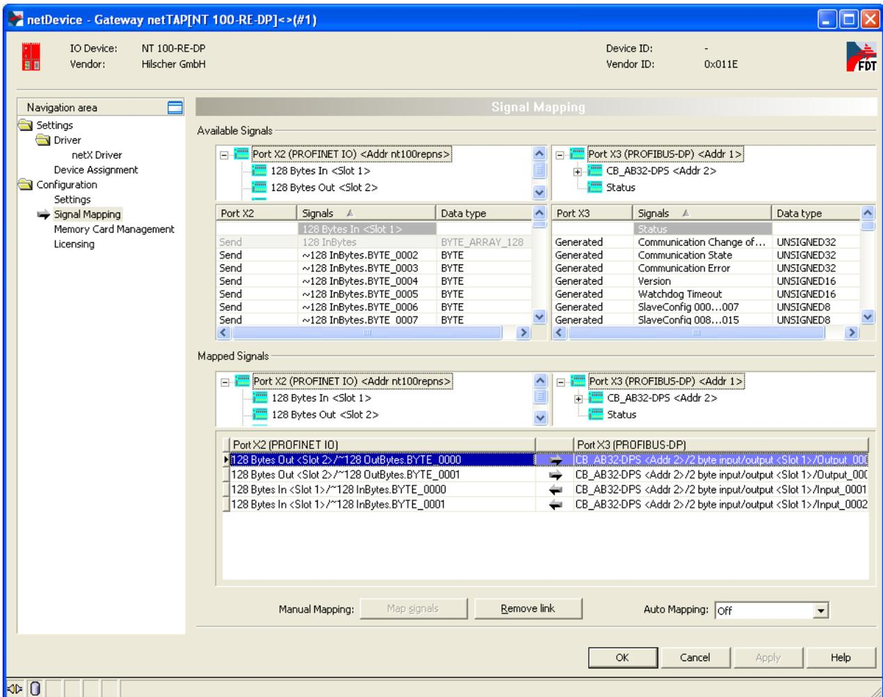
Figure 143: Signal Mapping
