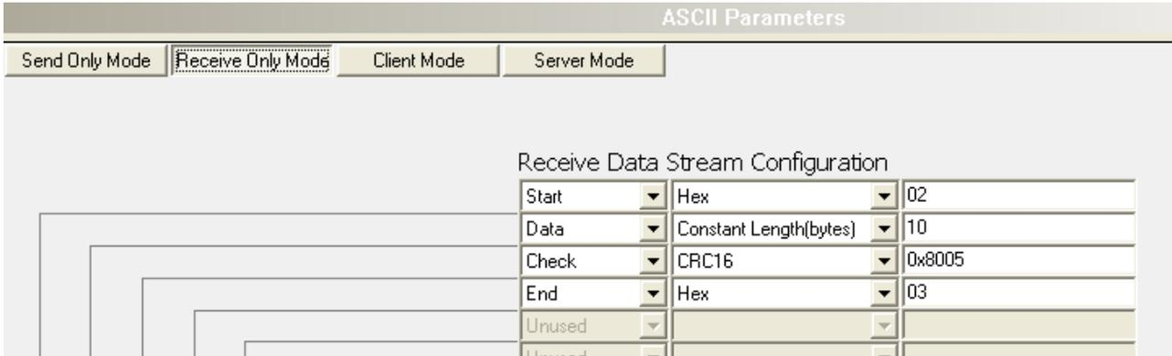
Table 67: ASCII Telegram Structure Example
