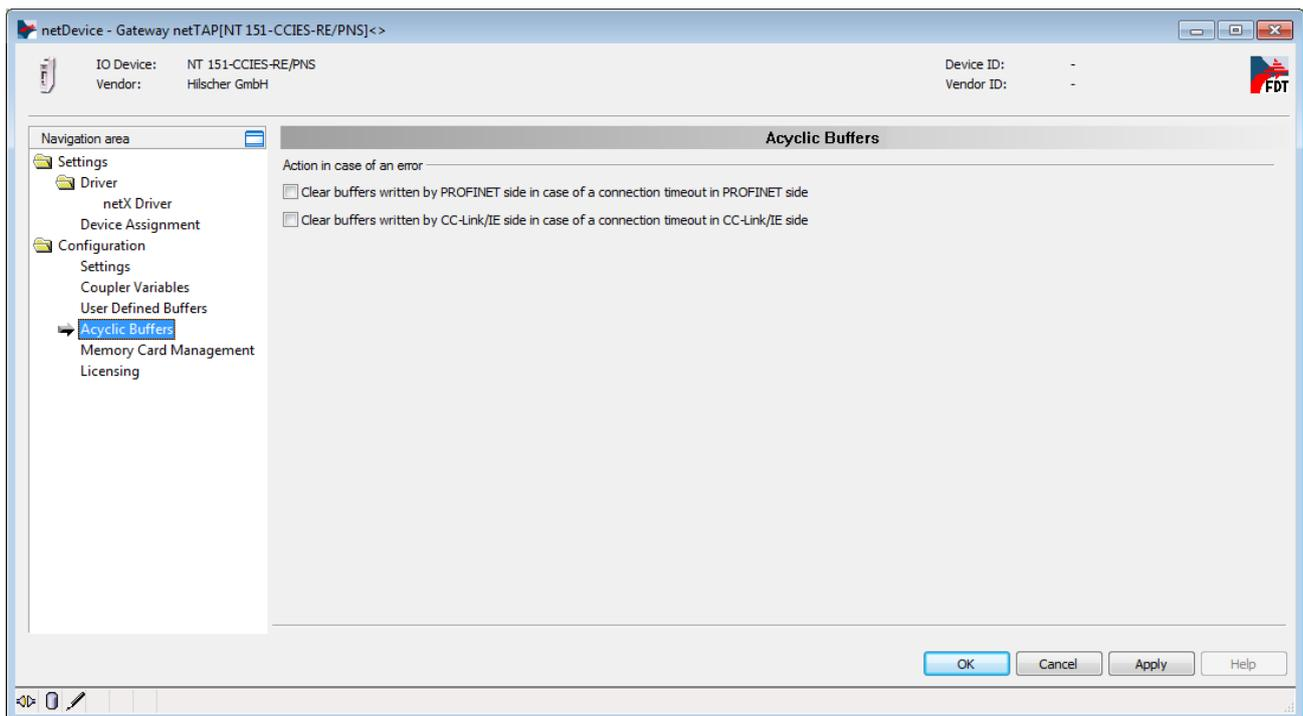
Figure 86: Configure Clearance of Acyclic Buffers in Case of Error
