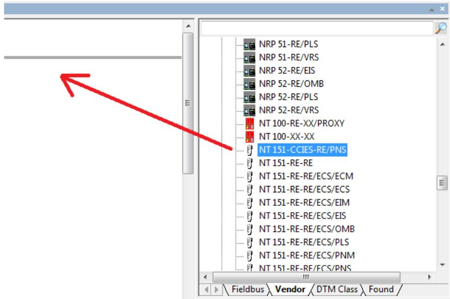
Figure 80: Insert Gateway Device into the Project
