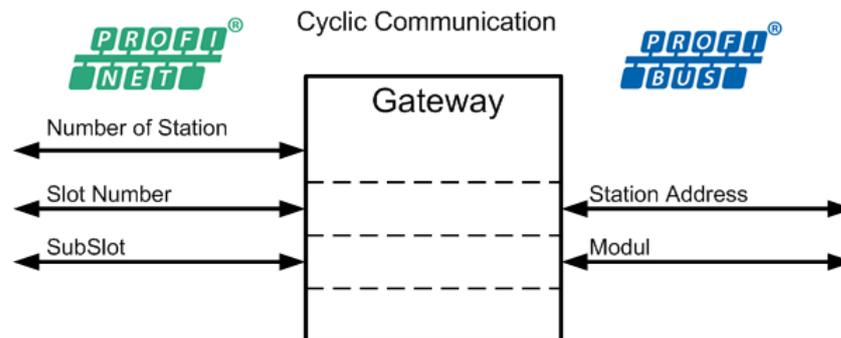
Figure 150: PROFINET – PROFIBUS Address Mapping
