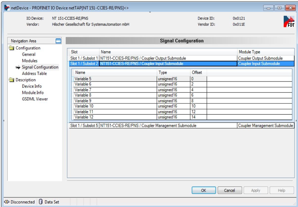
Figure 94: Signal Configuration dialog PROFINET IO Device
