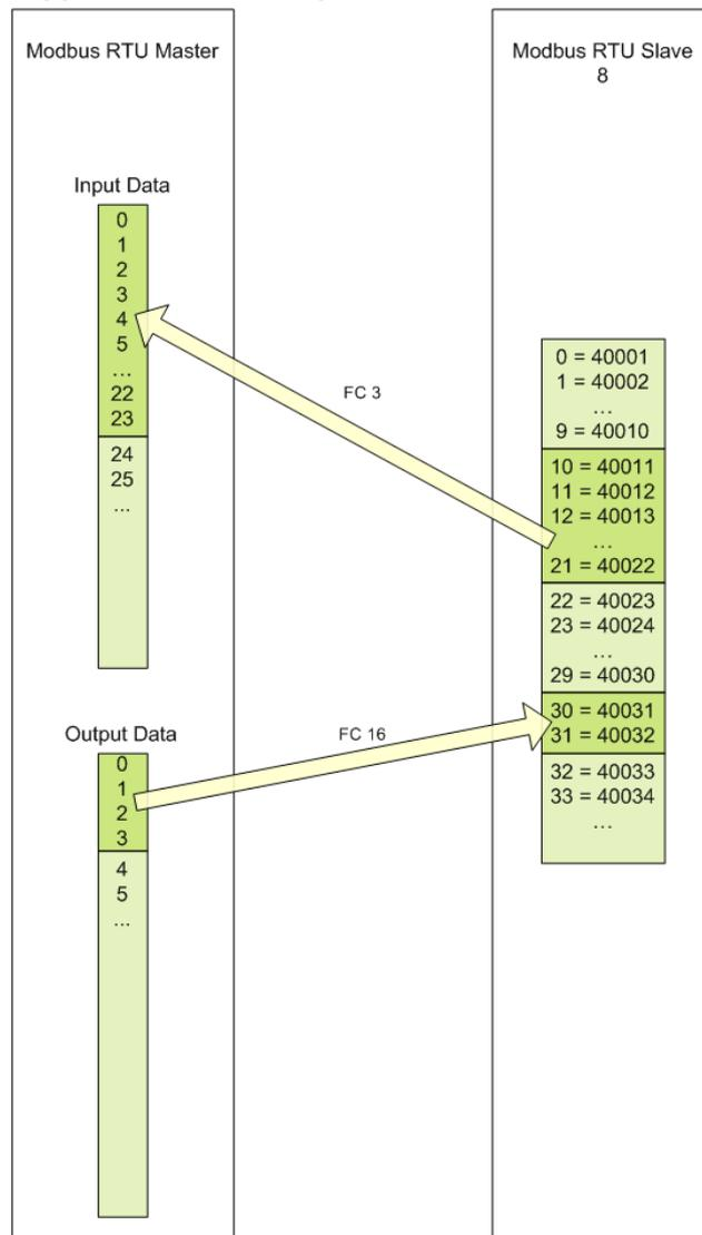
Figure 153: Examples - Reading Command with FC 3, Writing Command with FC16
