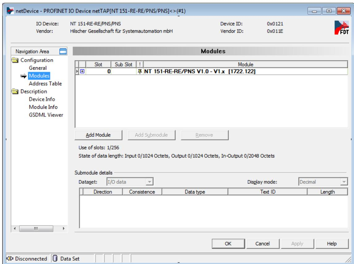
Figure 65: PROFINET IO Device Configuration Window
