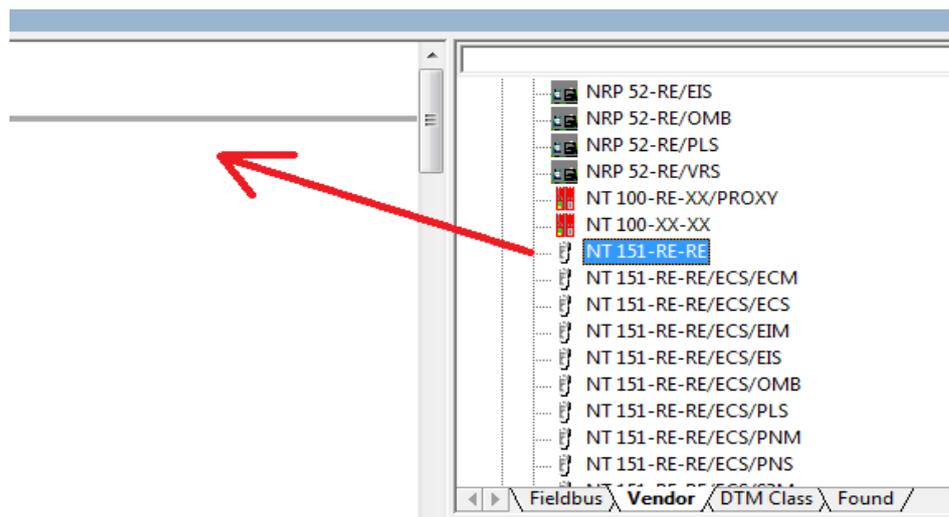
Figure 52: Insert Gateway Device into the Project
