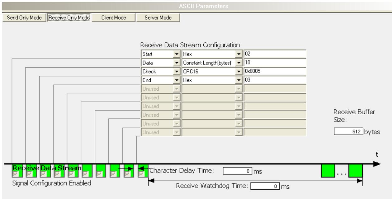
Table 75: Telegram Structure for the Operating 'Receive Only' Mode
