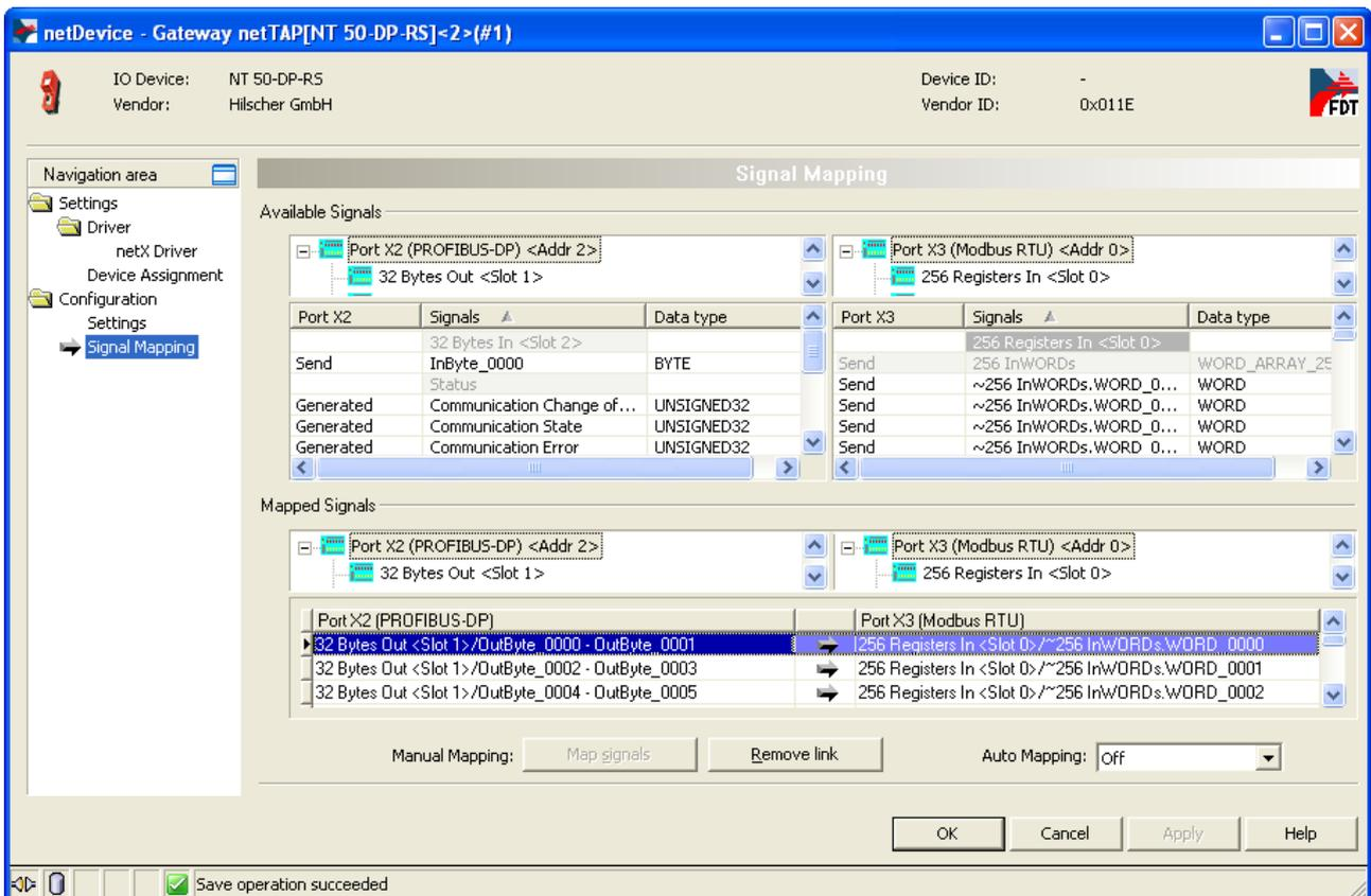
Figure 14: Gateway Signals mapped
