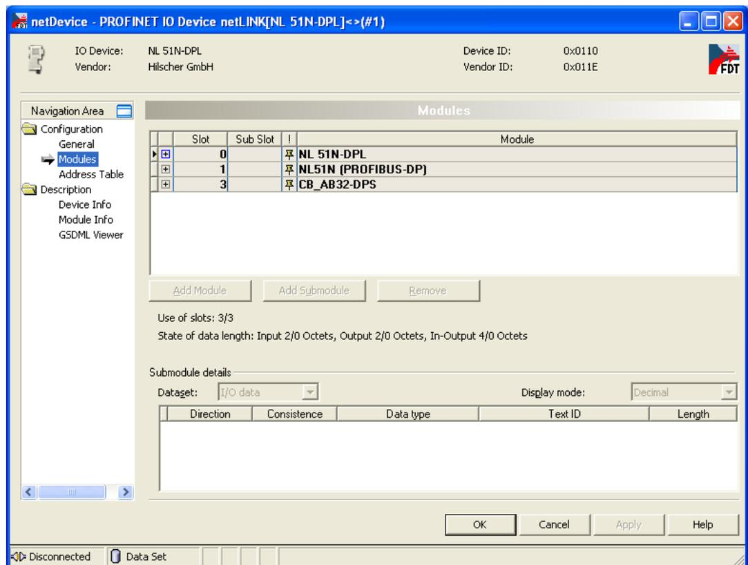
Figure 108: PROFINET IO Device Table
