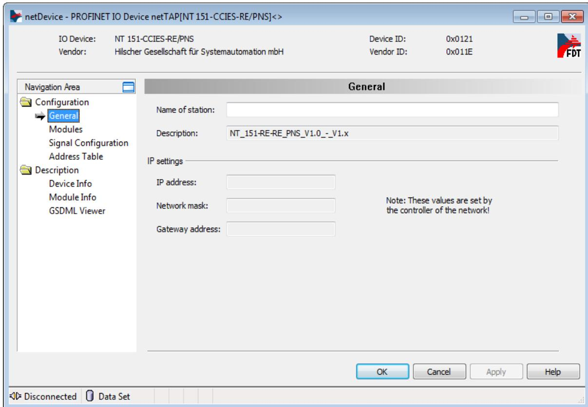
Figure 93: "General" Configuration dialog PROFINET Device
