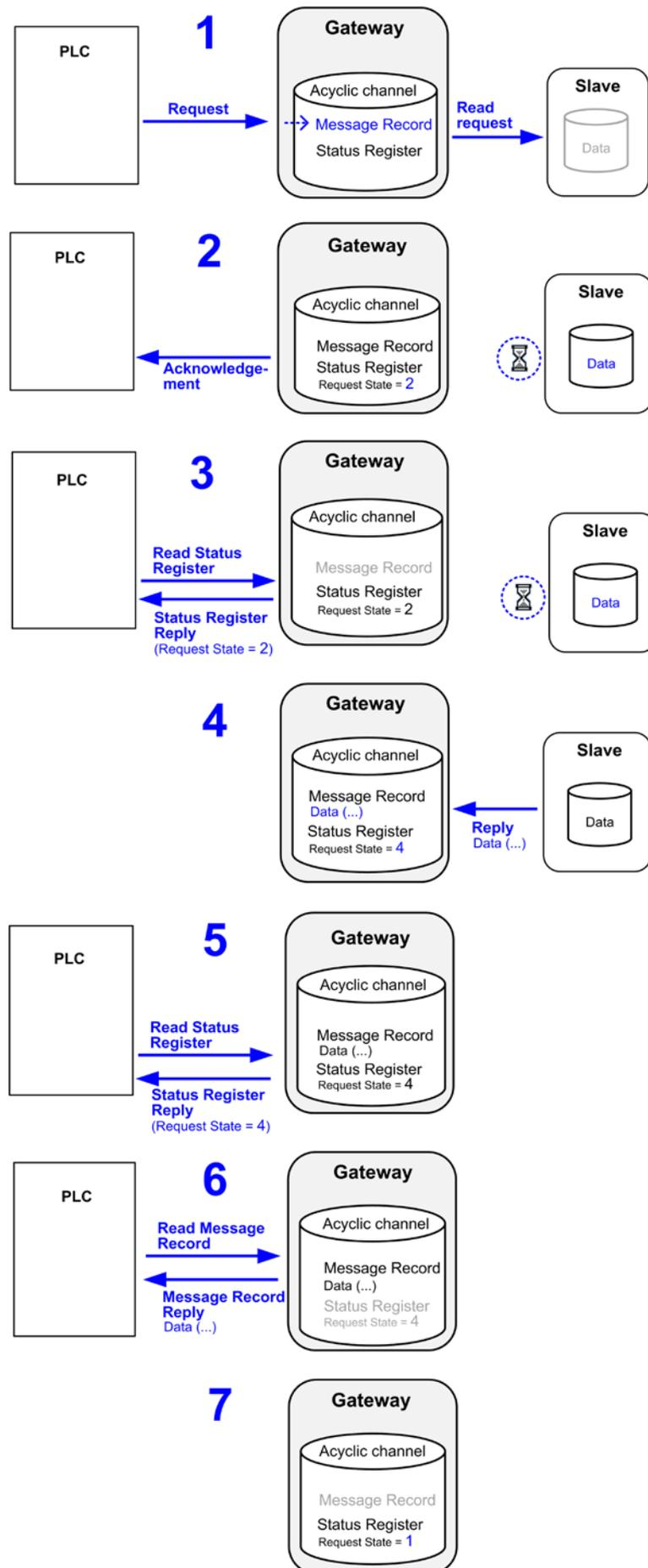
Figure 162: Sequence of Acyclic Reading Task
