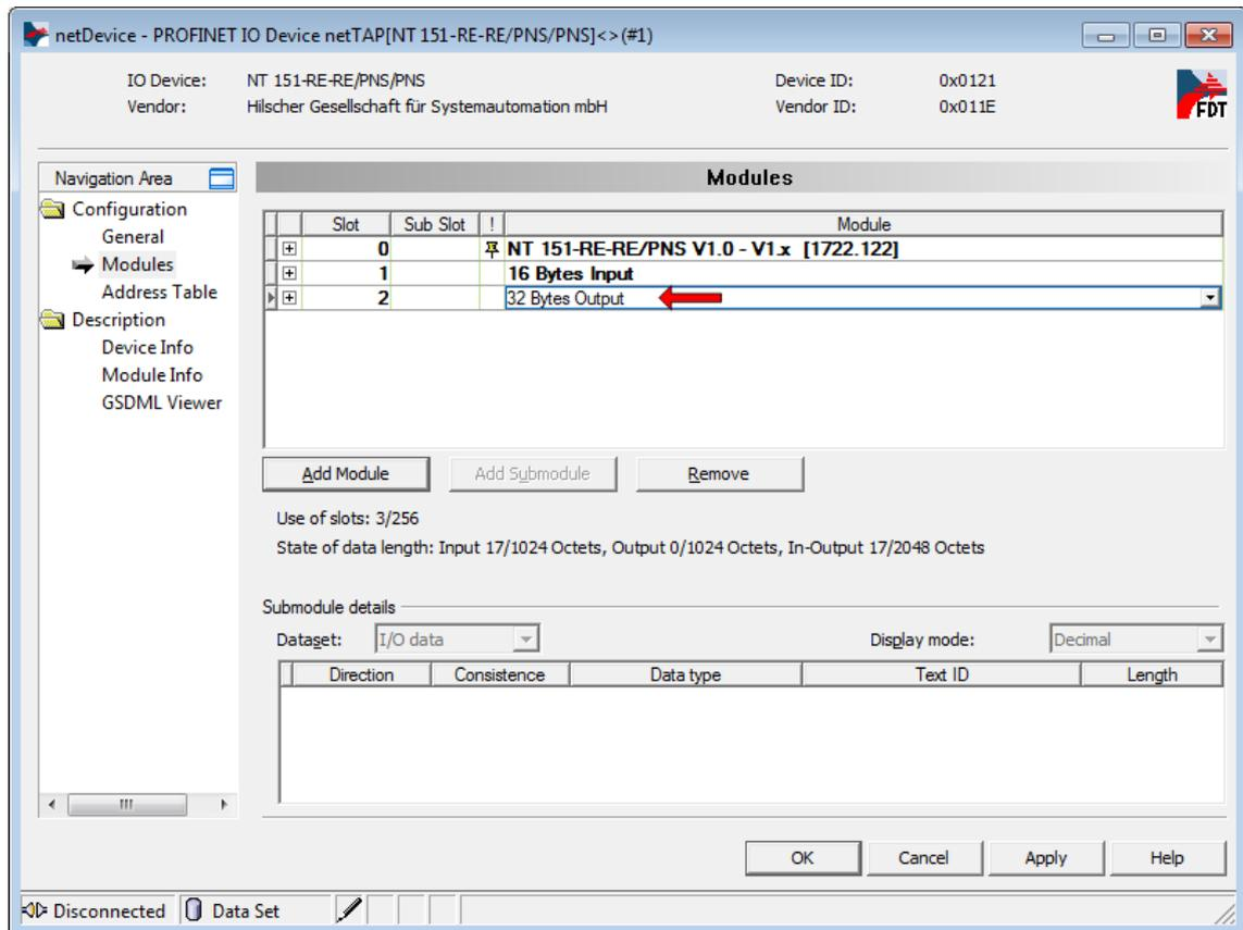
Figure 67: Configuring PROFINET IO Device at X3 (3)
