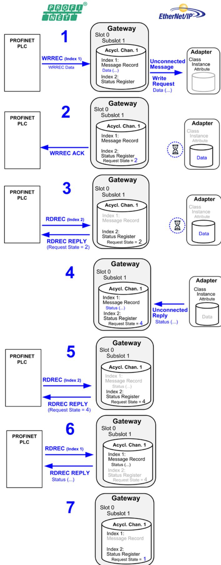
Figure 166: Sequence Acyclic Writing Task PROFINET to EtherNet/IP
