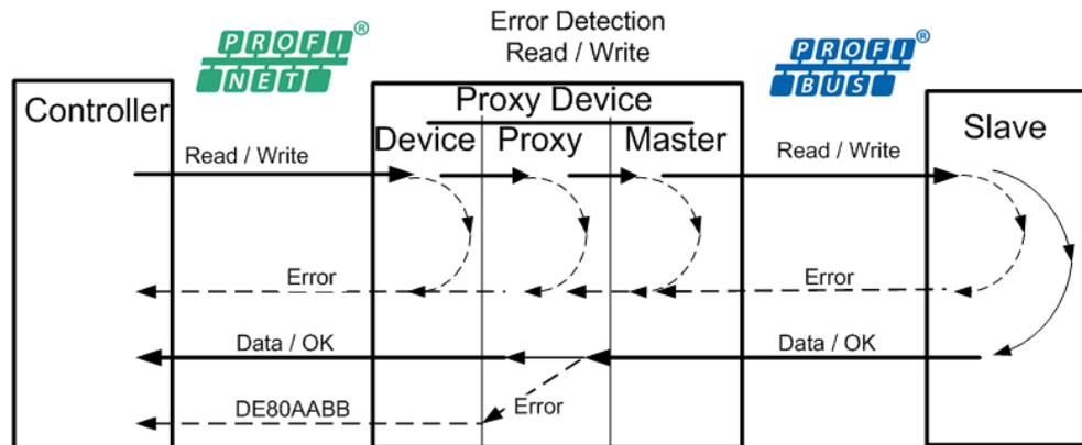
Figure 159: PROFINET IO – PROFIBUS DP Read/Write Error Detection
