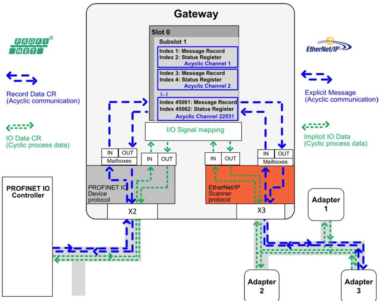
Figure 164: Acyclic Communication PROFINET IO-Device to Ethernet/IP Scanner
