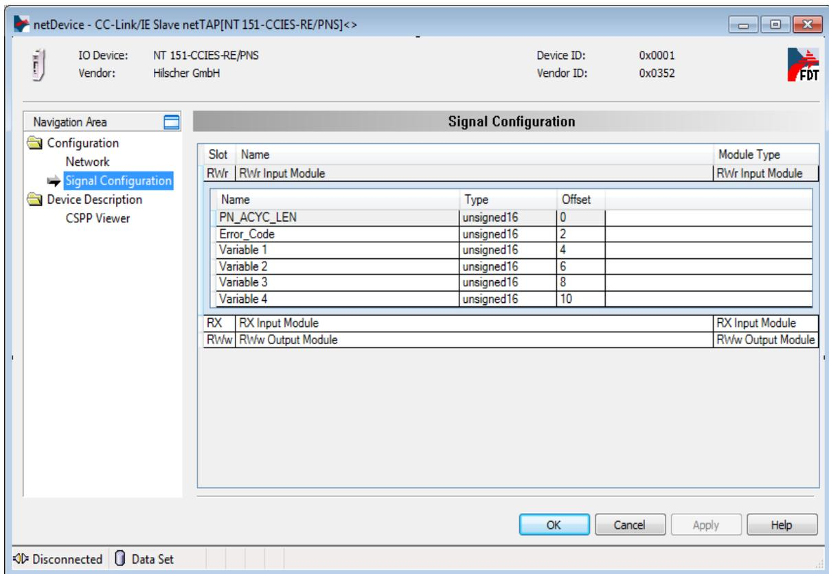
Figure 90: Signal Configuration dialog CC-Link IE Slave
