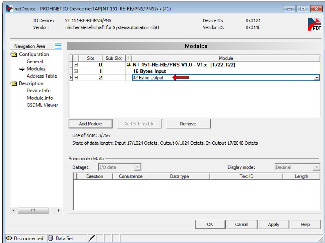
Figure 63: Configuring PROFINET IO Device at X2 (3)
