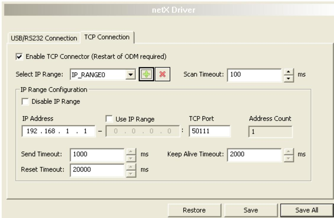
Figure 122: netX Driver > TCP Connection
