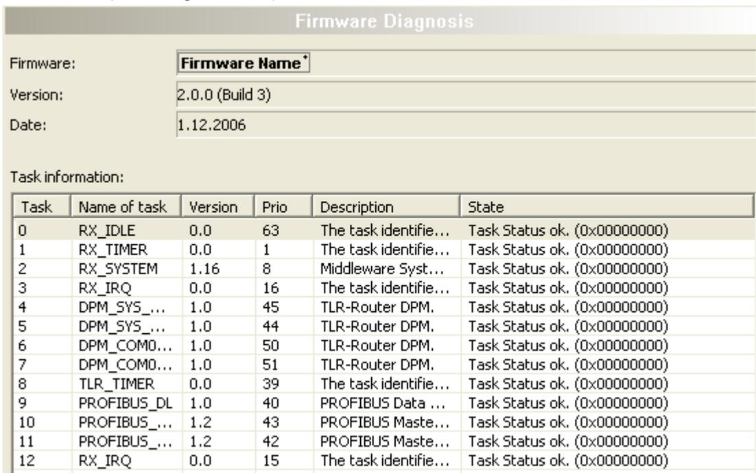
Figure 157: Firmware Diagnosis (\*The name of the Firmware is displayed.)
