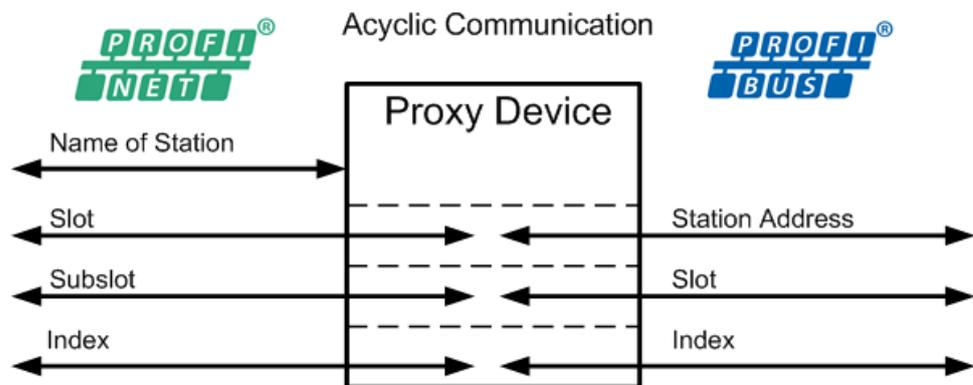
Figure 158: PROFINET – PROFIBUS Address Mapping
