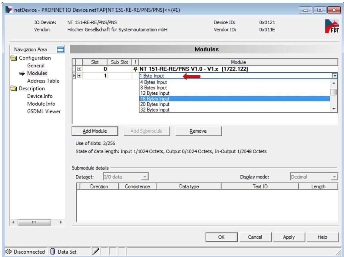
Figure 62: Configuring PROFINET IO Device at X2 (2)
