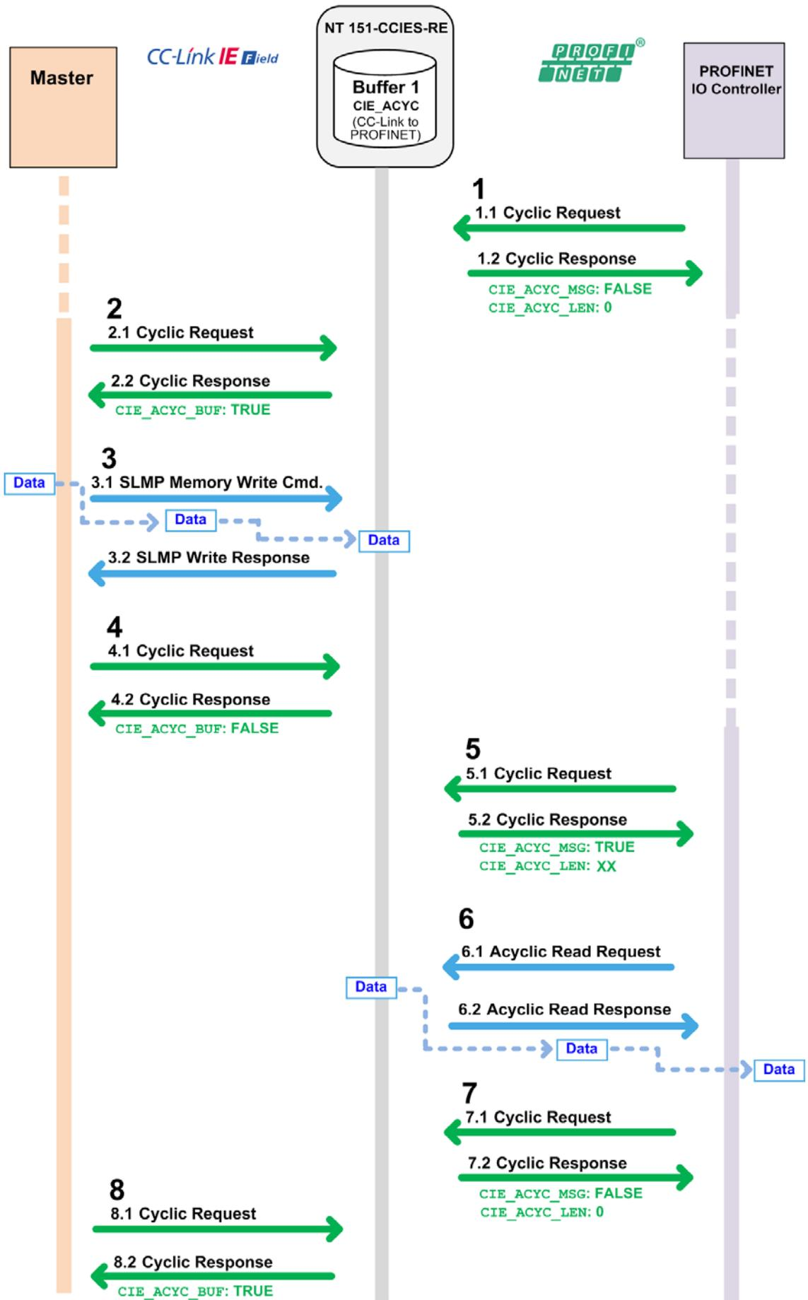
Figure 170: Sequence of Acyclic Communication of CC-Link IE Field to PROFINET
