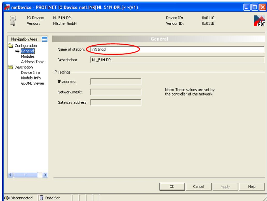
Figure 109: PROFINET IO Name of Station
