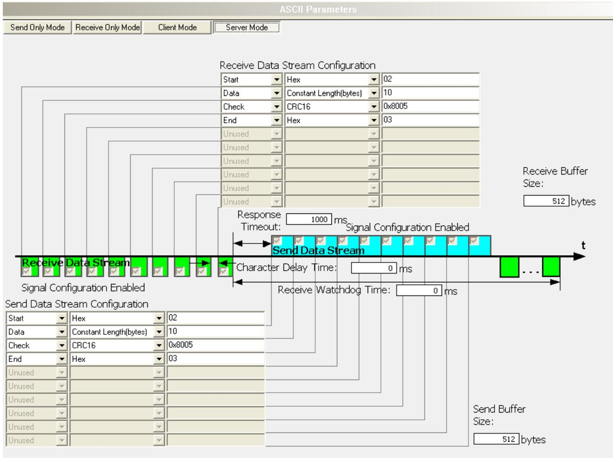
Table 79: Telegram Structure Parameters for the Operating Mode 'Server Mode'
