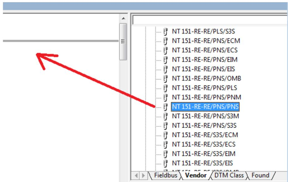
Figure 54: Insert pre-configured Gateway Device into the Project
